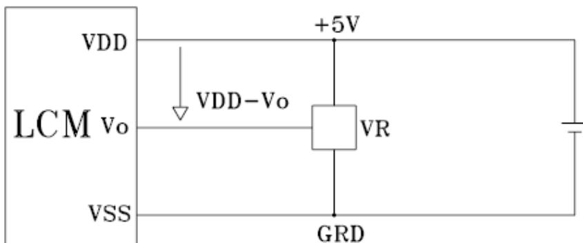
**VDD-Vo: LCD Driving Voltage**
