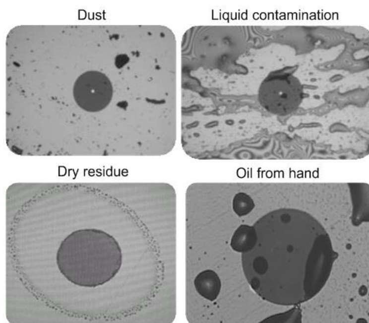
Figure 145: Appearance of various contaminants on a connector end face.
